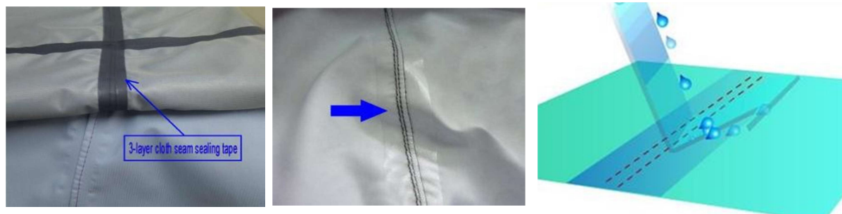
Fig-1. To prevent water from leaking through the seams
