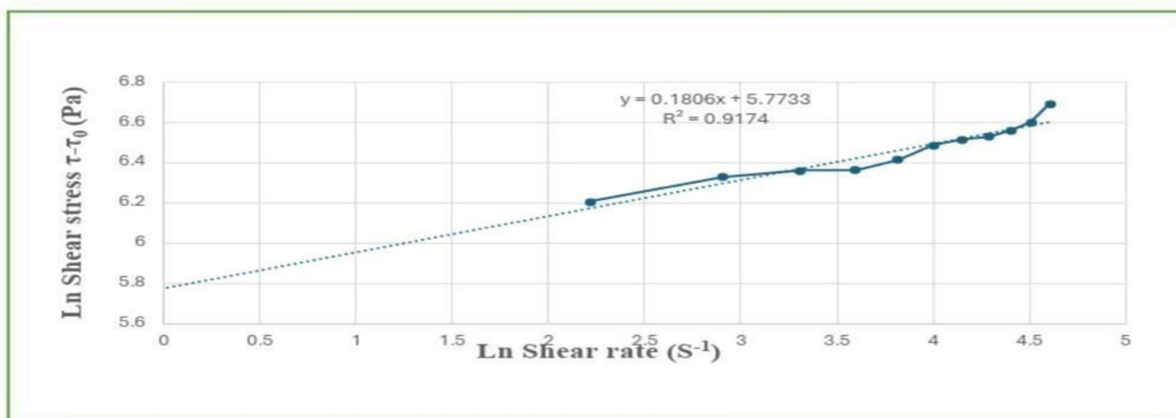
Figure 11. Linear plot between loge shear stress and loge shear rate of optimized formulation
