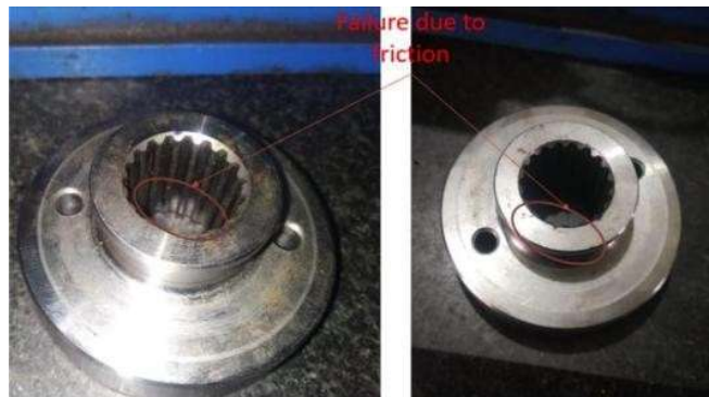
Failure due to friction
