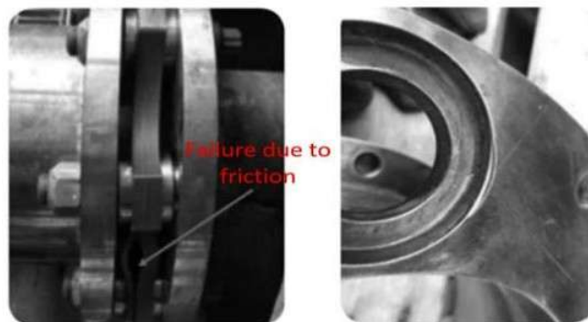
Fig.2 Failure due to friction with seal
